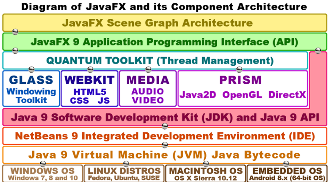
Figure 7-1. JavaFX Component Architecture from Scene Graph at the top down through Java, NetBeans, JVM, and OSs
